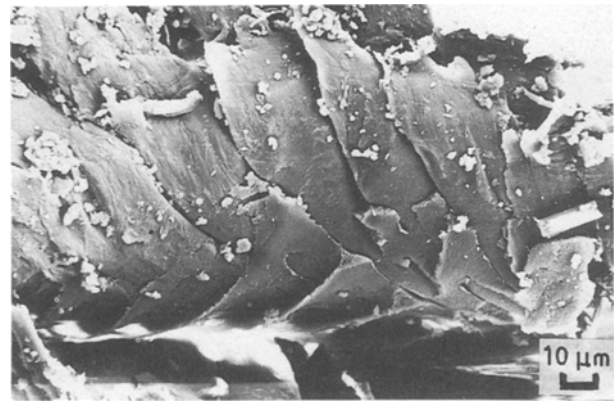
Figure 8 Chevron-like patterns in a resin-rich area in the carbon-Kevlar interface.
